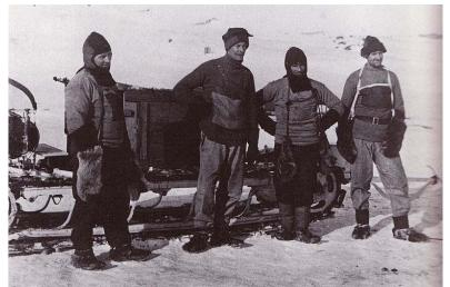
Figure 4: Motorized sled used on Scott's expedition. Three sleds were brought on the expedition. They all failed to operate after a short distance. (Source: Scanned from the book *Les Grands Explorateurs*. Herbert Ponting)
